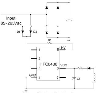
Figure 11: Start-Up Circuit
