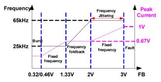
Figure 4: Frequency and Peak Current ( $V_{CS}$ ) vs  $V_{FB}$  Current-Mode Operation with Slope Compensation
