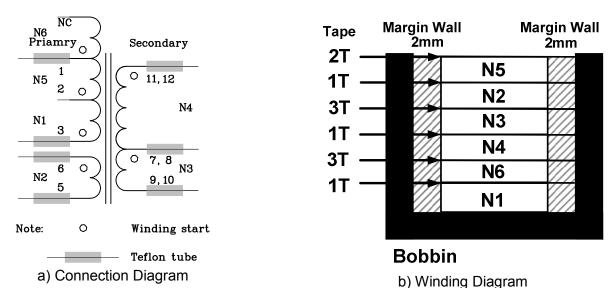
Figure 17: Transformer Structure
