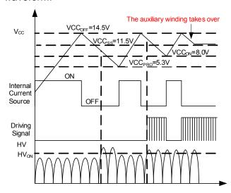
Figure 5:  $V_{\text{CC}}$  Under-Voltage Lockout The  $V_{\text{CC}}$  lower threshold UVLO drops from 8V to
