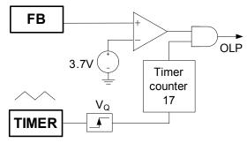
Figure 7: Overload Protection Block
