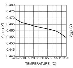
FB Level at which the **Controller Enters OLP** after Blanking Time
