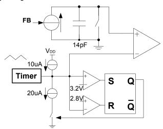
Figure 2: Frequency Jitter Circuit
