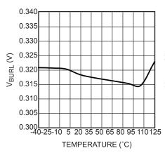
FB Level (Rising) at which the Controller Exits Burst Mode vs. Temperature
