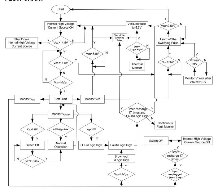
UVLO, brown-out, OTP & OLP is auto restart, OVP on VCC and Latch-off on TIMER are latch mode
