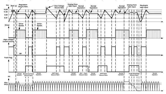
Figure 19: Signal Evolution in the Presence of Faults
