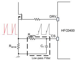
Figure 14: Low-Pass Filter on CS Pin
