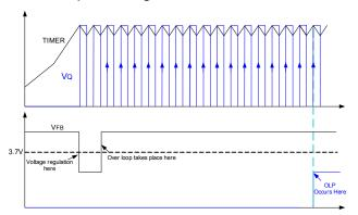
**Figure 8: Overload Protection**
