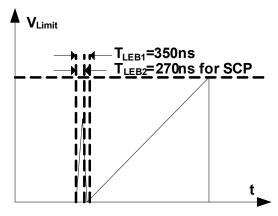
Figure 10: Leading-Edge Blanking
