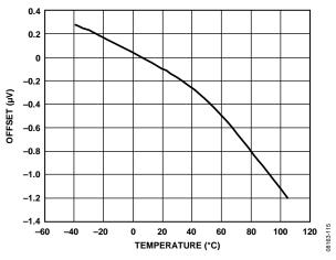
Figure 14. Offset Error (Gain = 128)
