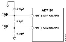
Figure 23. External Filtering Connections
