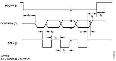
Figure 3. Read Cycle Timing Diagram
