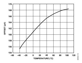
Figure 13. Offset Error (Gain = 1)
