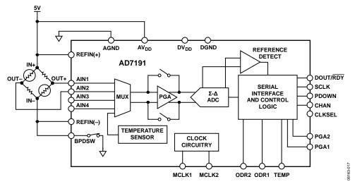
Figure 24. Typical Application (Weigh Scale)
