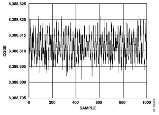
Figure 9. Noise ( $V_{REF} = AV_{DD}$ , Output Data Rate = 120 Hz, Gain = 1)
