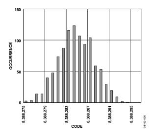
Figure 6. Noise Distribution Histogram  $(V_{REF} = AV_{DD}, Output Data Rate = 10 Hz, Gain = 128)$
