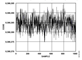
Figure 5. Noise ( $V_{REF} = AV_{DD}$ , Output Data Rate = 10 Hz, Gain = 128)
