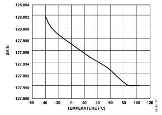
Figure 16. Gain Error (Gain = 128)
