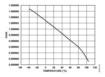
Figure 15. Gain Error (Gain = 1)
