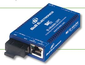
Measuring less than 3.5 inches deep and 2 inches wide, the IE-MiniMc Series converters are some of the industry's smallest copper-to-fiber media converters, with both data connections on the same side. The IE-MiniMc family of media converters are a fraction of the cost of other industrial grade alternatives. These products provide the ease and convenience of plug-and-play operation with features including Auto Negotiation and Auto-Cross.
