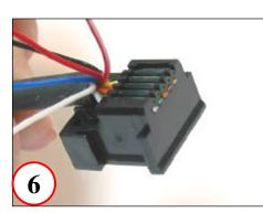
Trim lower row flush with front of load bar
