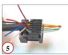
Place lower row conductors into load bar
