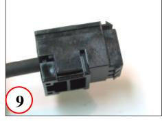
Place completed rear assembly into housing
