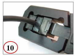
Place jack into crimper tool and crimp
