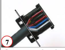
Snap upper row conductors into place. Cable jacket ends in front of square holes
