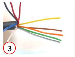
Align lower row conductors, fold upper conductors out of way
